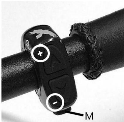
The gear shift is operated by pressing either a button on the Rohloff E-14 Switch Unit.
