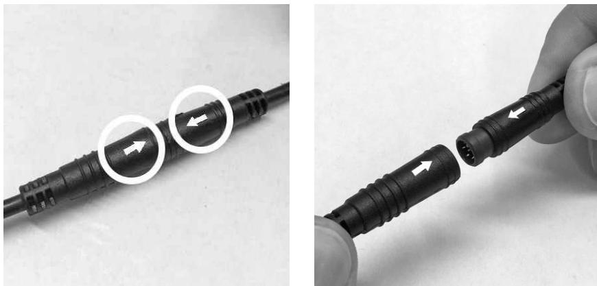
Both cable plugs are embossed with an arrow indicating their correct orientation.
