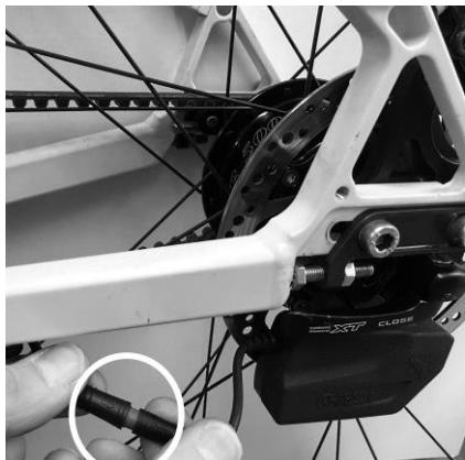
Re-connect the Rohloff E-14 Shifter Unit with the eBike System cable loom.
